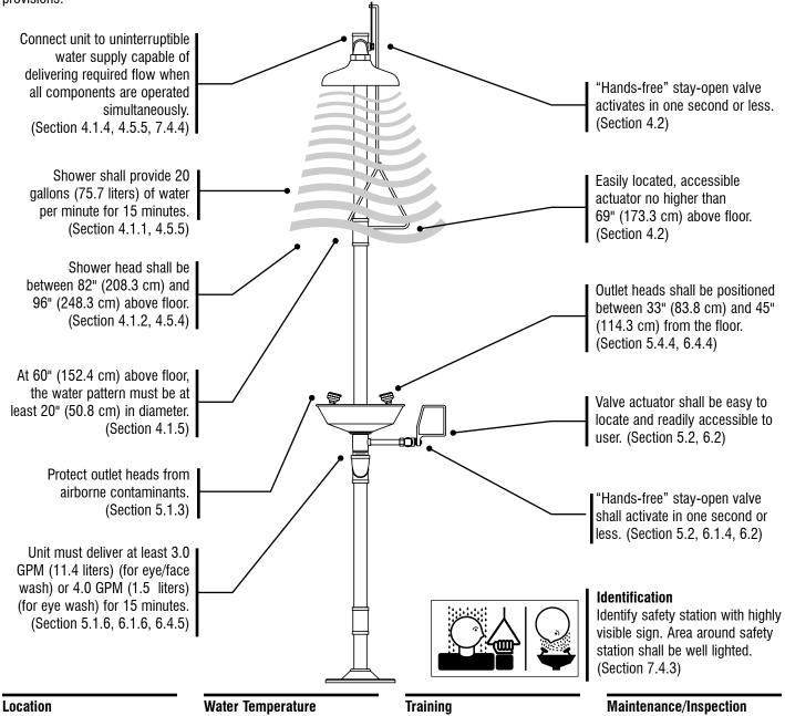
Install safety station within 10 seconds of hazard, on the same level as hazard and with unobstructed travel path. (Section 7.4.2)
